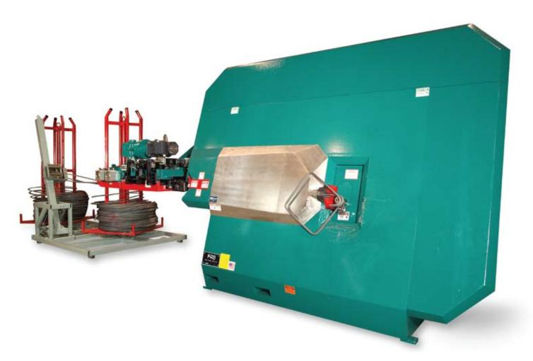
The Coil Form 1020 C ES processes dual strand #3 (10mm) through #5 (16mm) straight or coiled stock and single strand #6 (20mm) from straight stock. The Straightening system on this machine is controlled from the operator's station without the use of tools. The straightener rolls can be preset, recalled and changed with a push of the
